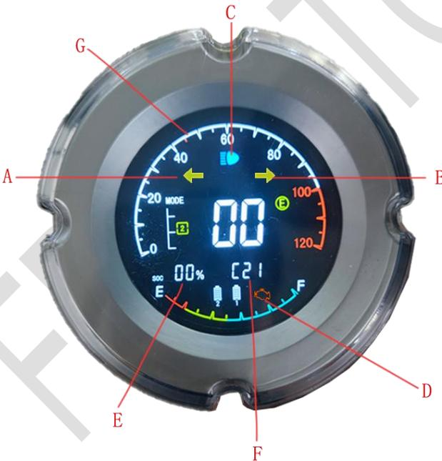
1. Battery SOC: the battery SOC% is controlled by CAN communication.
